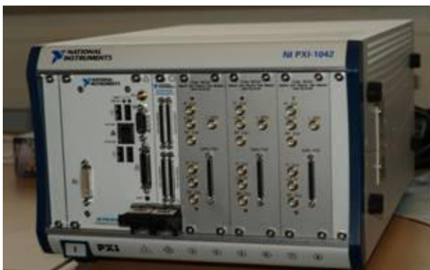
Figure 1: Relevant SAR/Galileo SAR-TB hardware on which GNSS simulator is based. The SAR-TB features custom PXI signal generator HW.
