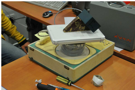
Fig. 7 – A 16 rpm Record Player to Impose a Constant Angular Velocity
