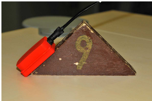
Fig. 3 – Woody Wedge for Coarse 45° Attitudes
