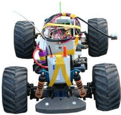
Fig. 6. Photo of buggy equipped with multiple sensors for enhanced tracking performance.
