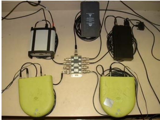
Figure 1: Zero-baseline test configuration to examine receiver hardware bias properties
