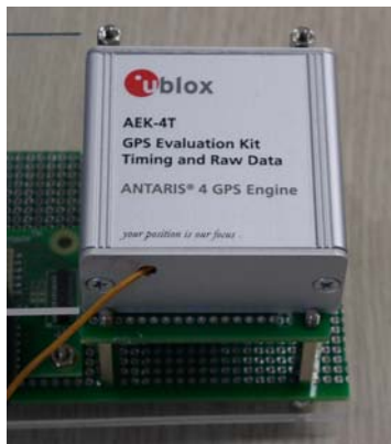
Fig. 6 u-blox AEK GPS Evaluation Kit
