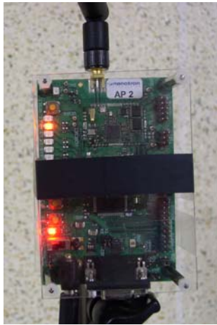
Fig. 5 IEEE 802.15.4a CSS nanoLOC Development Kit
